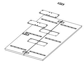
2) ATTACH THE CENTRAL BEAM TO THE TABLETOP a) Match the numbers on the central beam to those on the tabletop. Insert the M8x80 bolts with washers and tighten with a 6mm Allen Key.
