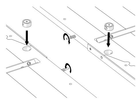
c) Push the two halves together, guiding the metal dowels into the Universal Connectors then tighten with an Allen Key.
